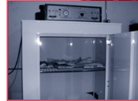
Dryer unit (left) dries electronic parts and papers.
